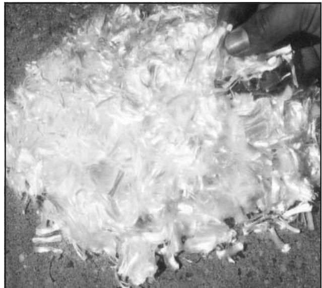
One type of synthetic fibers used in concrete
